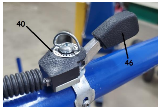
Figure Q: Throttle Control
