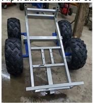
8.) Install frame tube into main frame, holes at coupler end face up & down, larger diameter bolt holes face up for the coupler.
