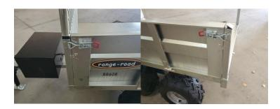
26.) Mount tailgate, put in 2 bolts and tighten until locknut plastic is engaged in the threads and go 2 more turns. Fasten lower clips.
