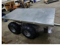
19.) Line up the tabs at the rear of the deck and insert the pivot bolts, tighten the bolts but leave space between the tabs nd frame so the deck can swivel up and down freely.
