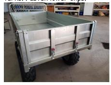
27.) Tighten the 3 bolts on front deck plate and the 2 bolts at the bottom of the rear corner posts.
