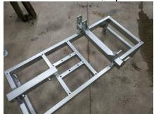
3.) Place the walking beams between the tabs on either side, there is not a right or left, either walking beam can be used for both sides, however, one leg of the walking bean is longer than the other, the 39cm leg of the axle should be towards the front of the trailer on both sides. Line up the hole in the walking beam with the tabs on the frame, push the pin in to hold axles in place.
