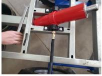
15.) Run the hydraulic hose trough the clips and bend the clips to hold the hose in place.
