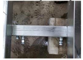
10.) Slide battery box onto frame tube and then slide the tongue jack on, install the 2 retainer bolts for the battery box but do not tighten, Move the tongue jack approximately 12cm back from coupler bolt hole and tighten the retainer bolt. (note battery box may be blue or black)
