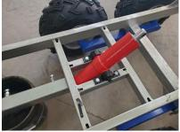
14.) Install the hydraulic hose onto the cylinder and tighten.
