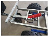
16.) Install the hydraulic pump into the battery box, check all nuts holding wires, overtightening can break the housing. 2 Bolts secure the pump through the bottom of the battery box.
