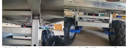
20.) Slide the battery box to approximately 15-20cm away from the deck and tighten the 2 retaining bolts.
