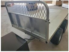
24.) Install rear corner posts into deck and put retainer bolts in, do not tighten yet..
