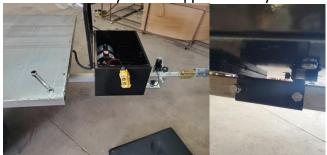
21.) Line up holes to mount the cylinder to the deck taba and insert pin, lock pins in place with circlip.
