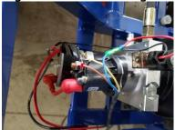
18.) Run the red, black and coated black controller wire along the frame using the clips to hold the wires in place, run the wires into the battery box and slide box into a position where the wires are long enough to attach to a battery and don't leave a lot of loose wire, tighten 2 battery box bolts to frame.
