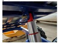
26.) Connect red & black wire to a battery, Operate switch to raise and lower tub 2 or 3 times, check Hydraulic oil level, add more if needed.
