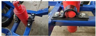
15.) Install hydraulic pump mounting 2 -16mm bolts from under the frame, use the supplied nuts as spacers to make sure the pump is held tight to the frame.
