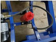
17.) Tighten all nuts holding wires, overtightening can break the housing.
