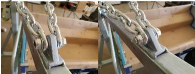
34.) Tighten bolt hold boom swivel into the locknut but not tight, swivel must be able to move,
