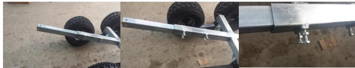
11.) Frame rail should extend approximately 40" passed main frame, tighten all 4 bolts and then all 4 nuts.
