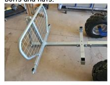
16.) Install outriggers and retaining handles.
