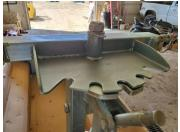
28.) Remove bolt holding winch cable roller, run winch cable through and re-install roller, tighten nut & bolt.
