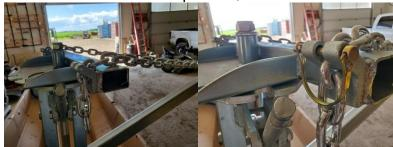
33.) Tighten bolt holding chains to boom.
