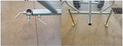
17.) Find hitch swivel and install to front of frame tube, tighten bolts, grease swivel with grease gun.
