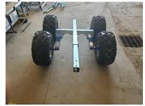
10.) Install 4 bolts with nuts into main frame.
