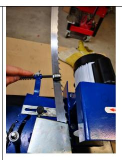
Slide the Right pressure wheel over the center of the blade
