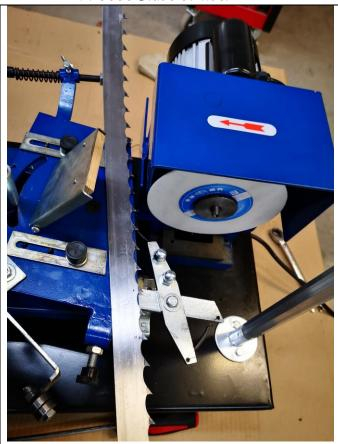
Once the blade is facing the correct direction, slide it towards the grinding wheel
