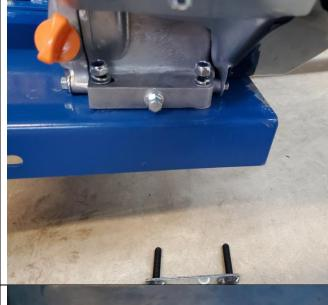
Once all 4 - 13mm nuts are threaded on, tighten them securing the engine into place.
