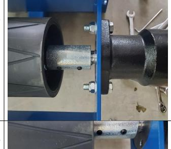
Mount the belt guides on each side of the rubber roller, leave a slight gap between the guide and the roller so they don't rub.
