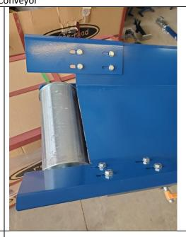
Install the belt and insert the pin into the lace to hold the 2 sections together.
