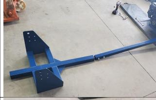
Remove the 2 - 16mm bolts  $\times$  17mm nuts, line up the holes in the 2 frame sections, reinstall the 2 bolts and nuts and tighten.
