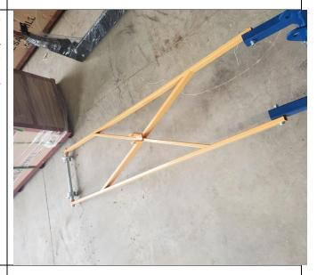
Remove the caps from the cylinder fitting and pull the rear cross frame down.
