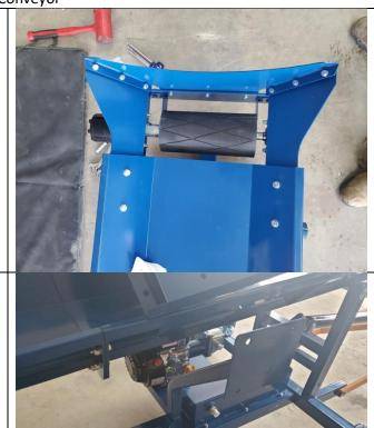
Insert the control valve arm and tighten the T-Handle.
