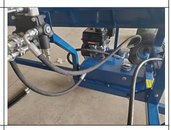
Plug the conveyor motor hoses into the control valve using the quick connect fittings.
