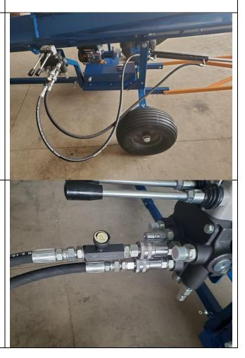
Install the suction hose between the tank and pump.
