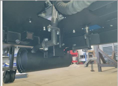
Fuel Tank Bracket can be installed. Can be done with the unit lifted or on the ground.
