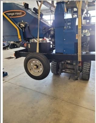
Install draw bar to the frame of the chipper
