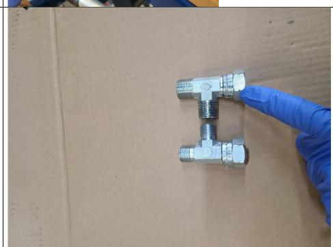
Showing the larger of the two "T's" that is to be installed onto the left side of the control valve.
