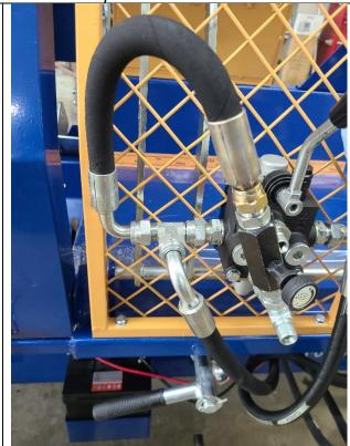
Locate the two longer hoses, already equipped with quick connects.
