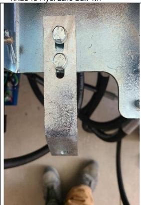
Loosely install the bottom bracket onto the swivel plate.
