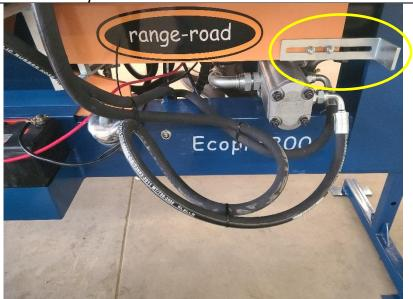
The control valve will now be prepped to install the hoses that go out to the cylinder.
