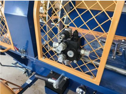
After the valve is loosely installed, the hydraulics can now be plumbed to the valve.
