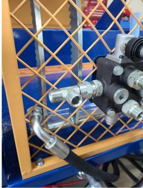
The hose that was originally taken off the pump will now be installed on the left port on the control valve (The port stamped with a "T")
