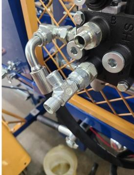
The 3/8' coupler with gasket will be installed onto the "T"
