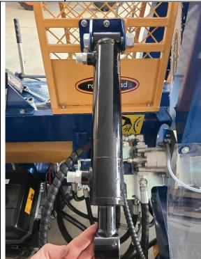
The large silver cylinder bracket will now be installed onto the lower bracket with the 2 provided nuts.
