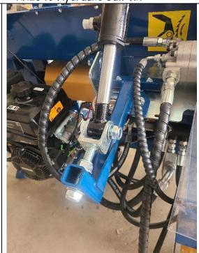
Remove the 2 plastic covers over the ports on the hydraulic cylinder.
