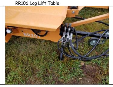
Connect the hoses according to the tags on the hoses..
