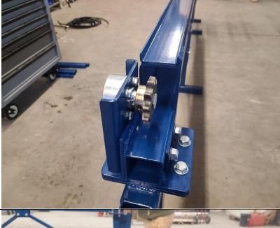
When installing the chain adjustment plates, run the long, tensioner bolt "in" to allow the adjustment gear to be as close to the rails as possible.
