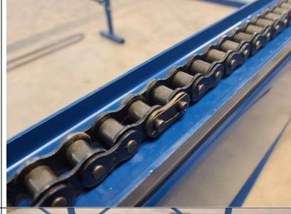
Run the tensioner bolts "out" to put tension on the chain.
