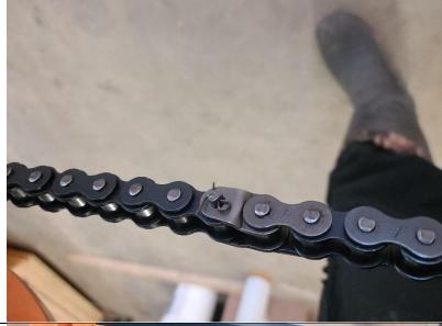
Now, put the chain back together by joining the open ends together.
