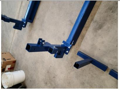
Picture showing the first lower leg being installed into the intermediate leg.
