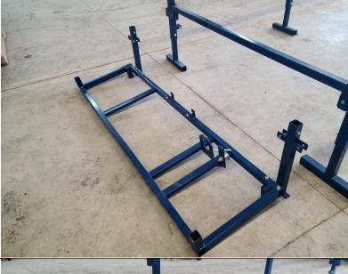
Ensure the tabs on the intermediate legs are facing lengthwise down the infeed, as shown here.
