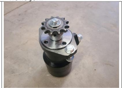
The hydraulic motor is installed with the ports facing down and the chain below the gear.
