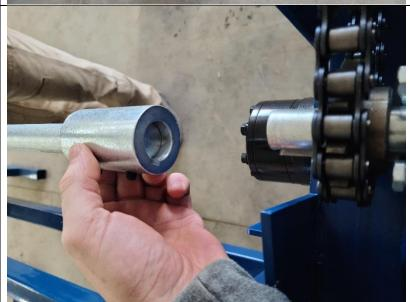
Install blue pipe over remaining silver shaft/coupler-then slide silver shaft into blue pipe as far as you can.
