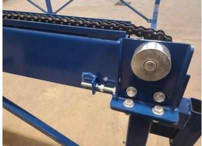
The drive bar will now be installed between the two halves of the table.
