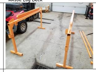
Insert the support leg into the drive roller bracket and then mount the drive roller bracket on the right side of the log deck. Add two of the rubber rollers and tighten the bolts.
