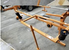
Install the hydraulic motor on the main drive bracket, do not tighten bolts.
