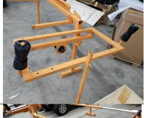
Insert the remaining front support bracket, and then slide the crossbar into the two support brackets.
