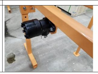
Insert the 2 round steel pipe ends in the drive sprockets. Tighten the allan screws. Install the pivoting log stops. Tighten the bolts so that the post can still easily move. Install the hydraulic pump side, close to the drive rollers and slide one of the 2 large chains onto the round steel pipe. Tighten the bolts. Slide the drive crossbar onto the round steel pipe, leaving the bolts loose.
