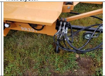
Connect the hoses according to the tags on the hoses.
