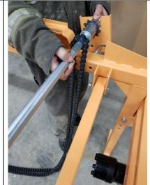
Position the chains so that you can insert the rear gear brackets for the chain to be connected. Insert brackets.
